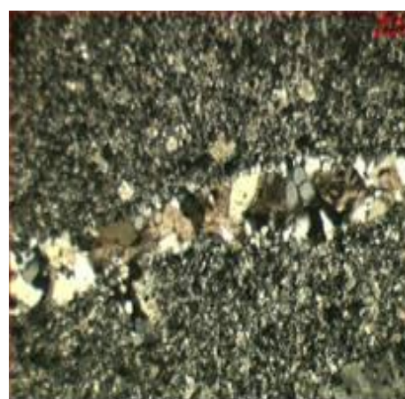
Fig 2 fracture filled by secondary quartz and carbonate
